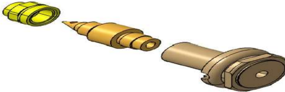
Figure 5.1 shows runner assembly models of hot runners
